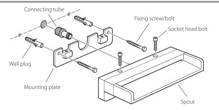
Before installing your new spout, flush through the pipework to ensure removal of debris, turn off the water supply.
