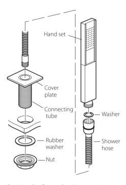
Position the Cover plate/connecting tube in place and from the underside slide on the rubber washer and nut. Tighten the nut to clamp on the cover plate.
