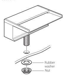
Position the spout in place, and from the underside slide on the rubber washer and nut. Tighten the nut to clamp on the spout.
