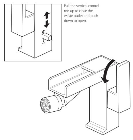
Moving the mixer lever forwards will actuate the flow of water and progressively increase the water temperature.
