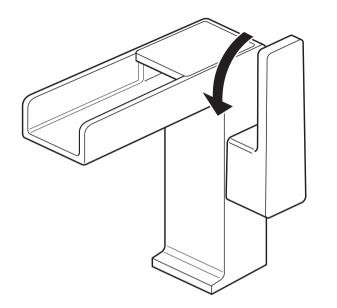
Moving the mixer lever forwards will actuate the flow of water and progressively increase the water temperature.
