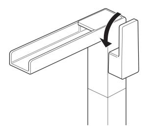
Moving the mixer lever forwards will actuate the flow of water and progressively increase the water temperature.
