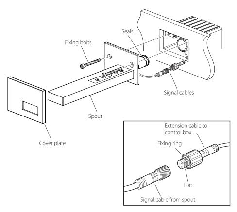
Flush through the pipe work to ensure removal of debris, turn off the water supply. Prepare the short extension coming from the control box to the spout, push through the hole in the side of the installation box making sure that the correct end is coming Line up the flats on both connectors and push together, screw on the ring to secure.
