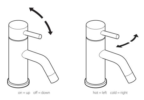
Moving the mixer lever upwards/downwards will increase/decrease the flow of water. Moving the mixer lever from right to left will increase the water temperature.
