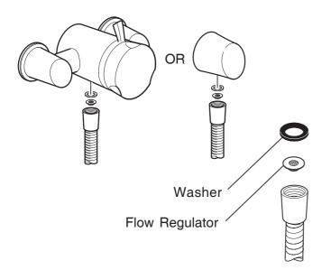
**Note!** If necessary, for high pressure systems, a 12 litre/minute flow regulator (supplied) can be fitted under the hose washer.
