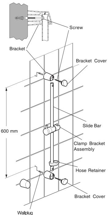
**1.3.** For solid walls drill two 8.0 mm diameter holes at 600 mm centres and insert the wall plugs.
