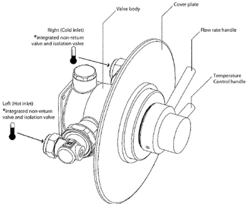
4. Ensure the valve is mounted to the correct depth from the finished wall surface. Make sure there is adequate clearance from the front to access all components and that the cover plate will cover the finished recess.
