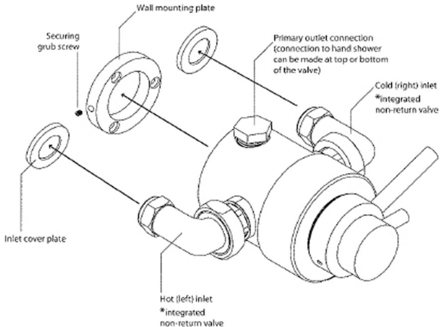
1. The valve body is designed to suit pipe work with centres of 152mm.
