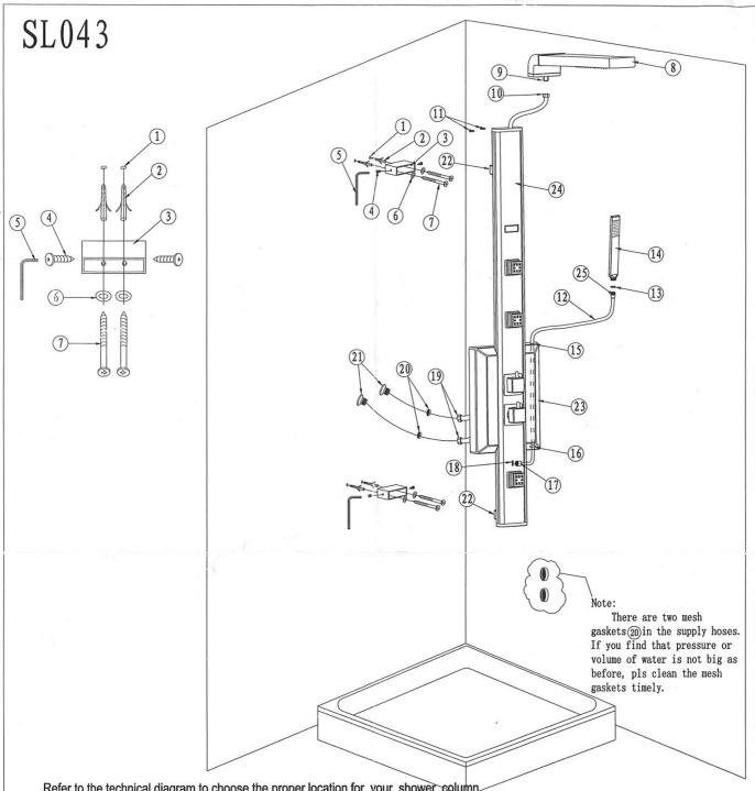
Refer to the technical diagram to choose the proper location for your shower column. You can adjust the column's vertical position based on the person's height. (Measurements given in the technical diagram are based on the average human height. 68 5/7").
