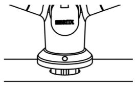
12. Once loosely in-place, check again that handle and spout movement is not obstructed.
