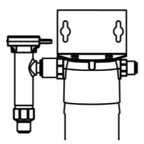
17. Screw the head bracket and the cartridge head (screws are provided for the bracket assembly) then screw the cartridge to the cartridge head after removing the yellow plastic protection cap. This simply pulls away.
