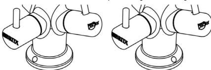
11. Position the tap onto base flange in desired position. Ensure all parts are located through the flange including the threaded clamping stud, single stainless steel flexible hose and the two plastic hoses all fit through hole in the base flange.
